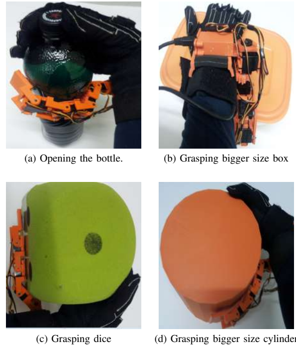
Fig. 3. Examples of tasks performed during the training with the supernumerary robotic finger.
