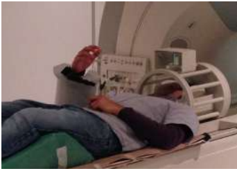
Fig. 4. The experimental fMRI setup: The subject is using MRI compatible finger inside the fMRI scanner.
